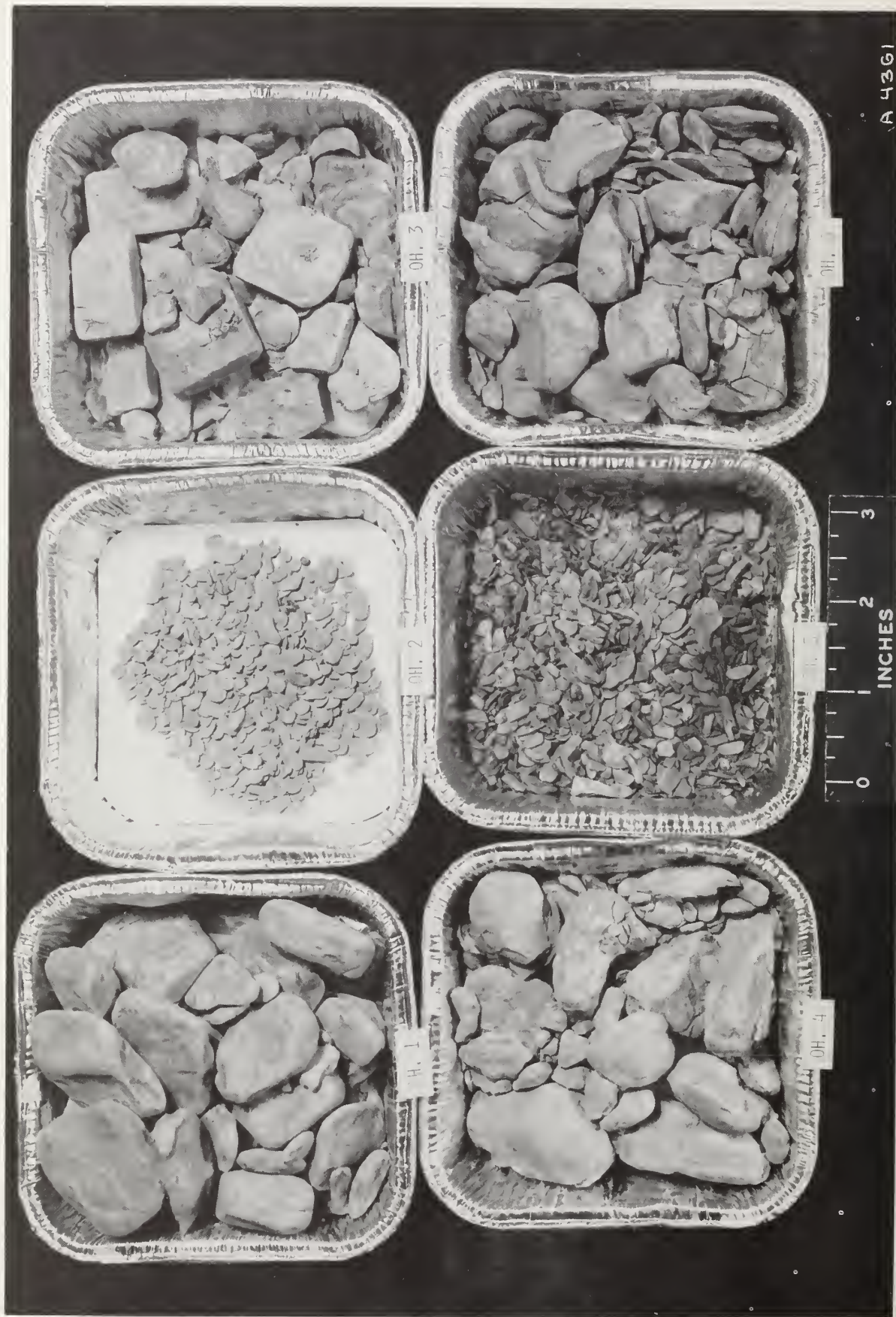
Figure 45. Material remaining after slake-durability testing, OH 1-OH 6.
